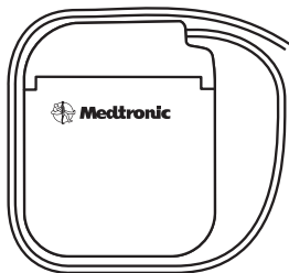
Figure 3. Wrap excess extension around the perimeter of the neurostimulator.
