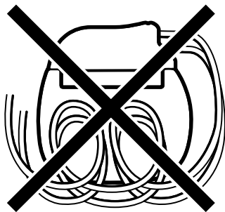
Figure 3. Wrap excess extensions around the perimeter of the neurostimulator.
